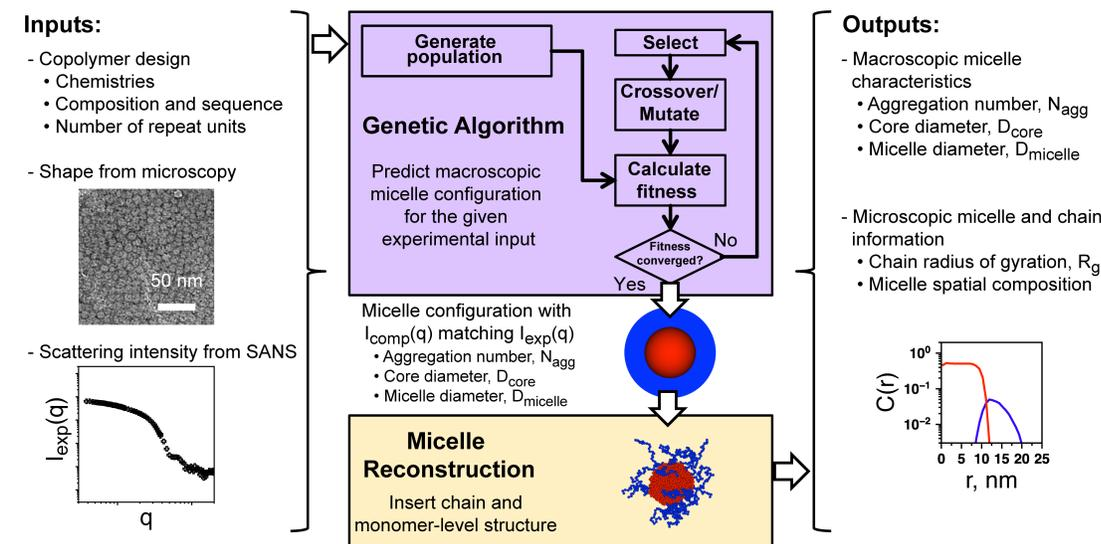
**Figure 1.** Work flow of CREASE process. CREASE will be combined with cryoTEM and SANS for particle characterization
